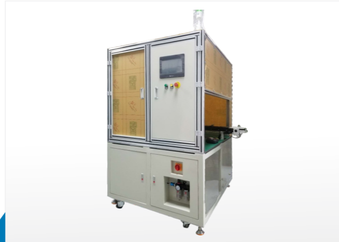
18650产线贴青稞纸机 18650 production line pasting highland barley paper machine
