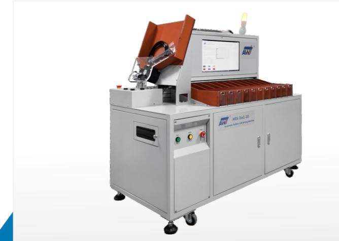
32650-18650兼容型自动分选机 32650-18650 compatible automatic sorting machine
