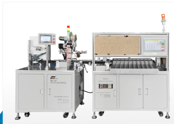
18650自动贴青稞纸+分选对接一体机（一字型） 18650 automatic barley paper paste + sorting and docking machine (in-line type)
