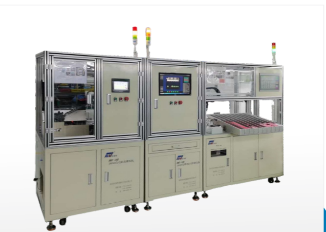
18650自动贴青稞纸+CCD检测+分选一体机 18650 automatic highland barley paper + CCD detection + sorting machine
